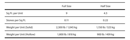
The Servian Wall is typically used as a gravity wall as there is no intrinsic interlock between units. However, when the hollow units are used, Cast-in-place concrete (with or without rebar) can be used to fill the cavities and lock the units together.
