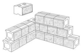
Place first Corner unit so small face will be hidden behind the final construction.
