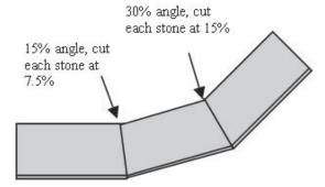
For gradual curves, units can be cut as required. Again, it is recommended that both units be mitred at 1/2 the total angle so that the units sit flush together.
