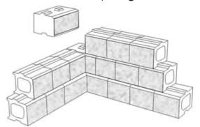
Place first Corner unit so small face will be hidden behind the final construction.
