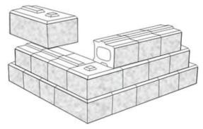
1st Course– Position corner unit so both rough faces will be exposed in the final construction.
