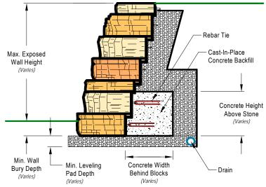
See Project Specific Design Drawings for Full Construction Details
