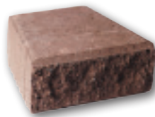
COPING UNIT 200mm deep x 225mm (tapered to 150mm) wide x 100mm high (7.87" deep x 8.9" (tapered to 5.9") wide x 3.93" high)
